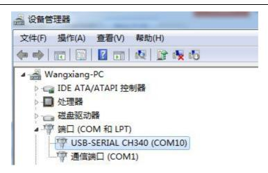
As shown in the figure above, your serial port number is COM10 at this time, please remember this serial port, you need to fill in this serial port number in the sensor monitoring software.
