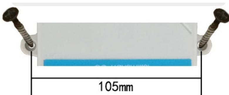
The wall-mounted “王”-shaped shell is wall-mounted. The installation holes are located in the middle of both sides of the device. The installation hole diameter is less than 4mm, and the hole spacing is 105mm. It can be installed with 3mm self-tapping screws.
