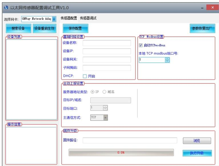
The software interface is divided into the following parts, as shown in the figure, the left side is the device search and operation information display area, and the middle is the configuration area, which can carry out basic device configuration, sensor debugging and firmware upgrade.
