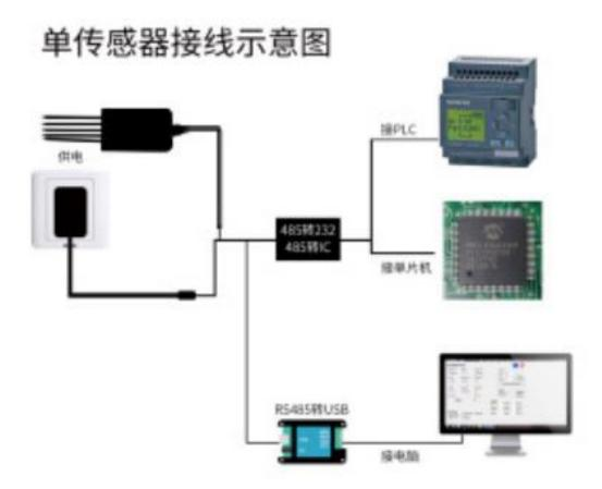
This product can also be used by multiple sensors combined in a 485 bus. In theory, one bus can connect more than 16 485 sensors. If more 485 sensors are needed, more 485 devices can be expanded using 485 repeaters. The other end is connected to the PLC with 485 interface chip through 485 interface chip, or can be connected to the computer by using USB to 485, the sensor configuration tools provided by our company to configure and test.
