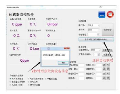
Then click on the connected device to get sensor data information in real time. If your device is a gas concentration sensor, please select "Gas Concentration Sensor" at the sensor type, "Formaldehyde Transmitter" for the formaldehyde sensor, "Analog Transmitter Module" for the analog transmitter, and
