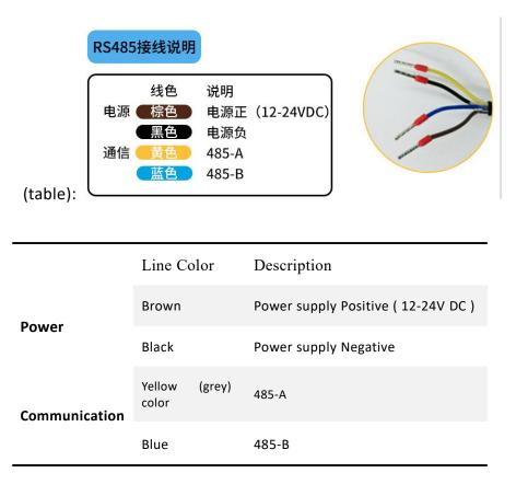
Note: Please be careful not to connect the wrong wiring sequence, the wrong wiring will cause the equipment to burn down.
